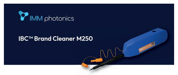
Patented fiber optic cleaner (US Conec) for cleaning 2.5 mm connectors such as SC, FC, ST for UPC and APC connectors. The cleaning pin turns while the cleaning band is drawn over the fiber end surface. This ensures that the fiber end surface is left clean after a single cleaning operation.
